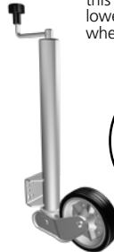
Clamp for height adjustment and fixture of the jockey wheel
